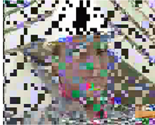
Algorithm III (MVEA) - Encrypted sign bits of DCT coefficients and Motion Vectors (FOREMAN Frame#101) w/ fixed 127-bit key
