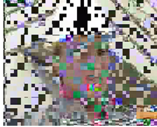
Algorithm II (VEA) - Encrypted sign bits of DCT coefficients (FOREMAN Frame#101) with fixed 127-bit key
