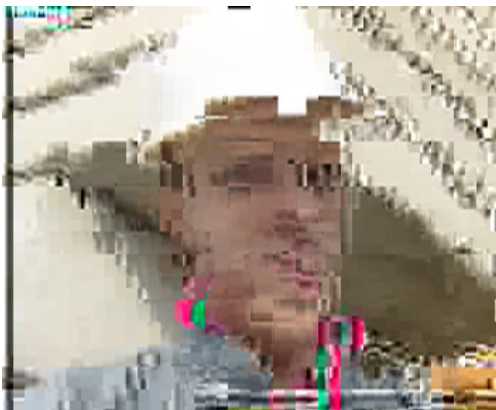
Algorithm III (MVEA) - Encrypted sign bits of DCT coefficients and Motion Vectors (FOREMAN Frame#101) with fixed 64-bit key
