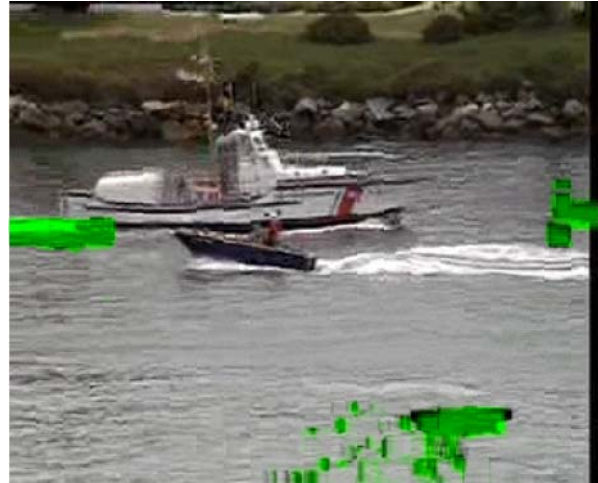
Figure 3: B-Frame #65 from "coastguard" stream showing propagation of errors. Y PSNR: 17.538345
