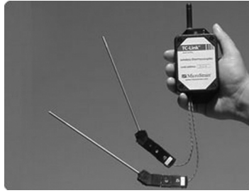
FIGURE 20.5 TC-Link TM wireless thermocouple system. (Source: www.microstrain.com/TCLink.htm )
