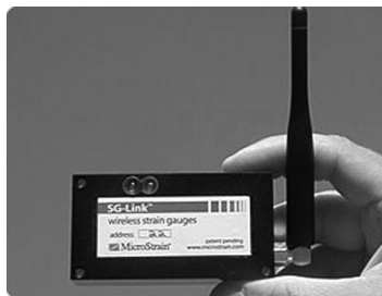
FIGURE 20.4 SG-link™ wireless strain gauge system. (Source: www.microstrain.com/SG-link.htm )
